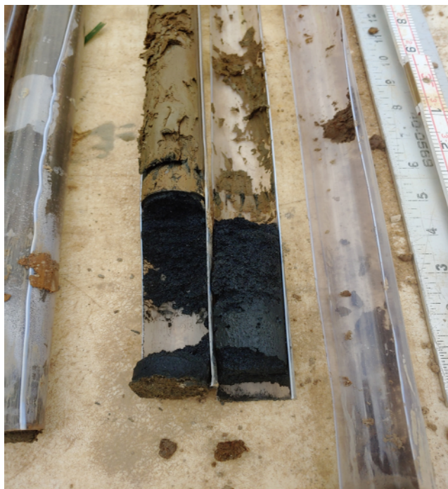
Evidence in Geoprobe sample of petroleum release.
